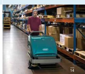
Optimized SweepMax Plus dust control system offers higher customer productivity with less dust going to the filter resulting in fewer shake backs and more time spent sweeping. The SweepMax Plus cyclonic system offers excellent indoor and outdoor dust control and helps reduce cost to clean, improve facility image, and provide a safe environment.
